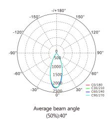
All luminous intensity values shown radially from centre are in cd. Elevation angle values are shown around the outside of the graph.
