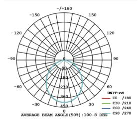
All luminous intensity values (shown radially from centre are in cd. Elevation angle values are shown around the outside of the graph.
